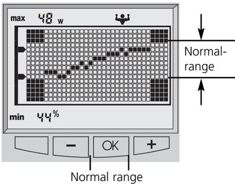
The normal range calculated for each person is shown in the trend display by the range between the fields in the corners.
